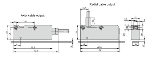
Permissible tolerances for reading head mounting
