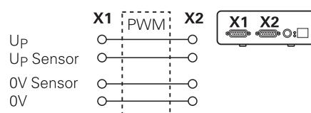
Example 2 – The device powers the encoder via X1:
