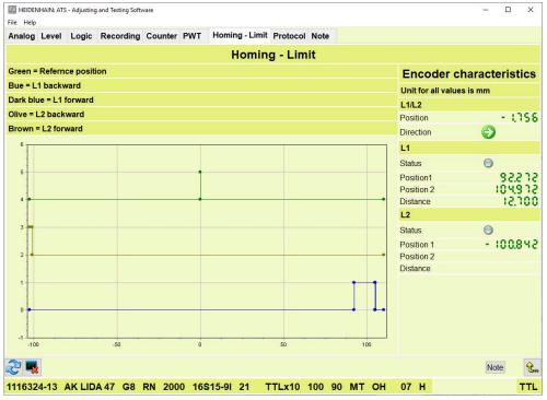
Figure 74: Homing - Limit view of the Incremental signal function
