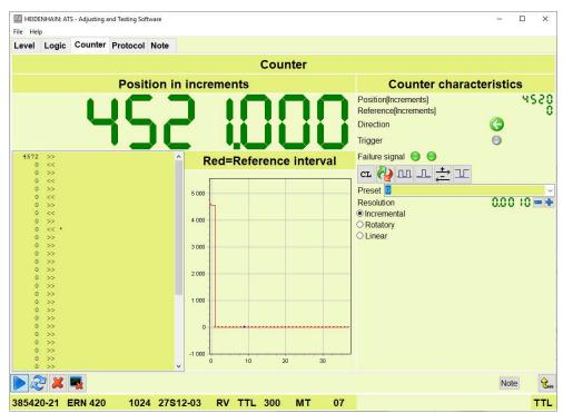
Figure 71: Counter view when examining an encoder with one reference mark
