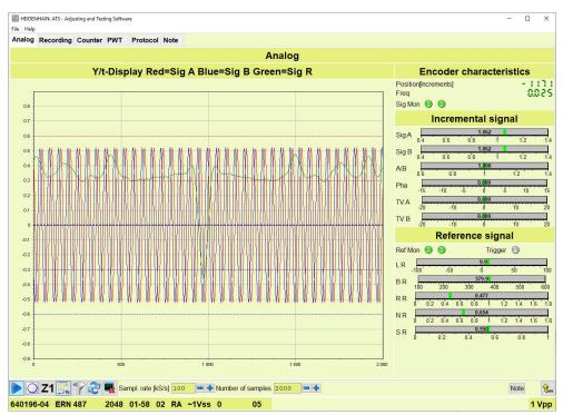
Figure 38: Incremental signal function with reference signal
