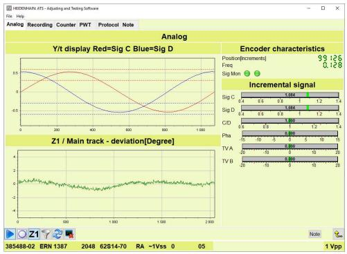
Figure 40: Y/t graph and Z1/Zn graph when checking the commutation signals C and D
