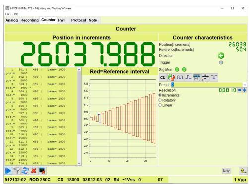
Figure 53: Display after the nominal increment has been determined
