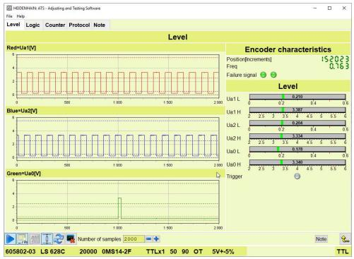
Figure 64: Incremental signal function when evaluating the reference signal
