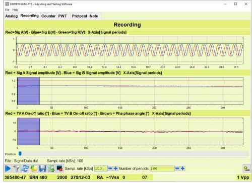
Figure 45: Recorded signal periods without error
