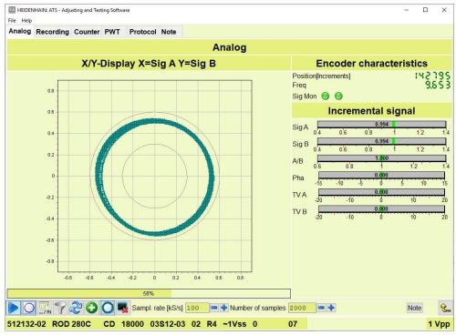
Figure 32: X/Y diagram with active persistence
