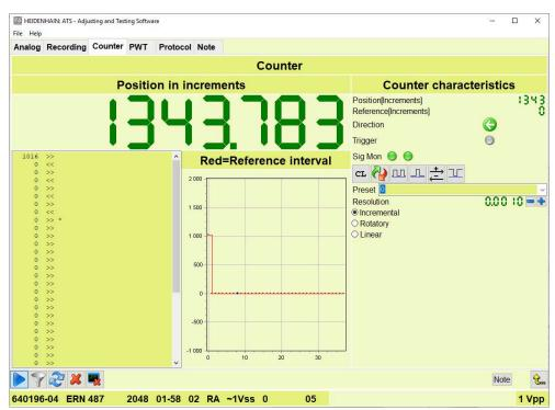
Figure 51: Counter view when examining an encoder with one reference mark
