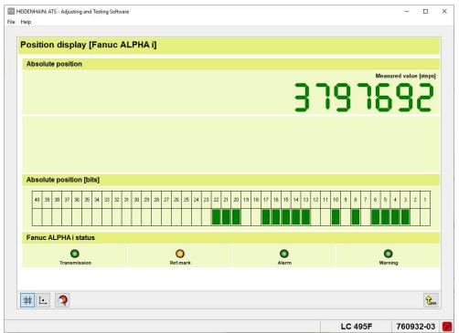
Figure 146: Position display function
