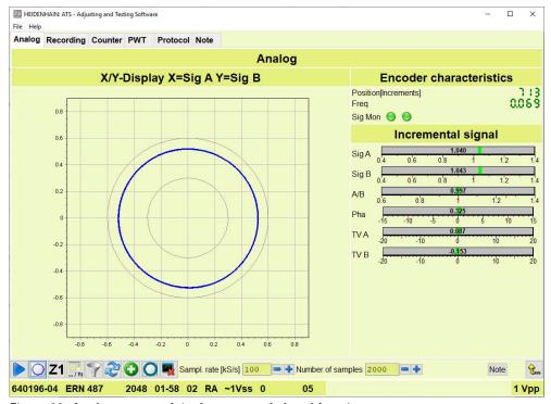
Figure 29: Analog screen of the Incremental signal function
