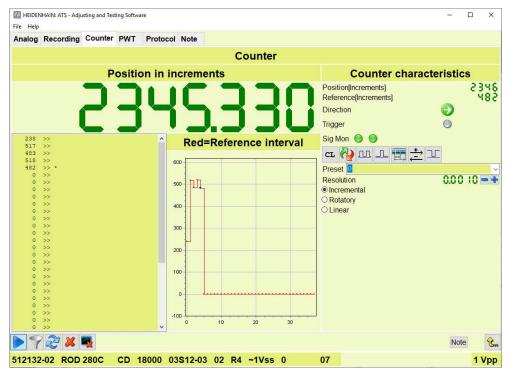
Figure 52: Display during determination of nominal increment
