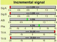
Measurement results are within the tolerance limits
