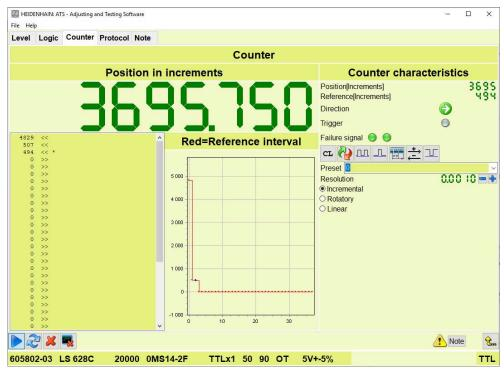
Figure 72: Display during determination of nominal increment
