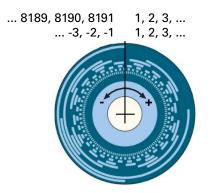
Figure 84: Counter limit of a 13-bit rotary encoder
