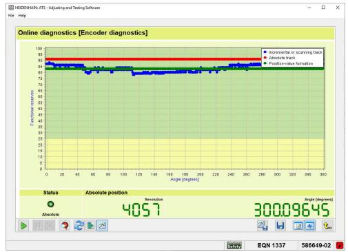
Figure 105: Result of the online diagnostics in the X/Y display
