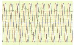
Figure 36: Complete reference pulse including quiescent value and usable component
