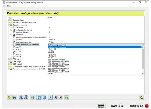
Figure 134: Temperature sensor type connected parameter in the encoder configuration
