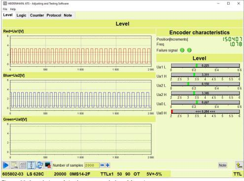
Figure 62: Level view of the Incremental signal function
