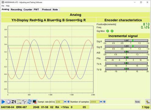
Figure 30: Analog view with Y/t graph
