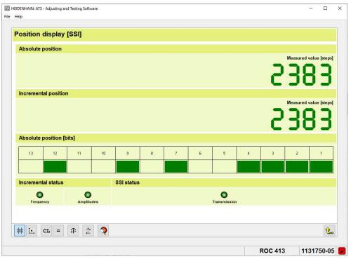
Figure 152: Position display function
