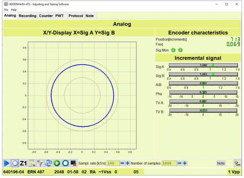
Figure 26: Analog screen of the Incremental signal function
