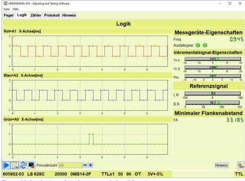
Figure 65: Logic view of the Incremental signal function
