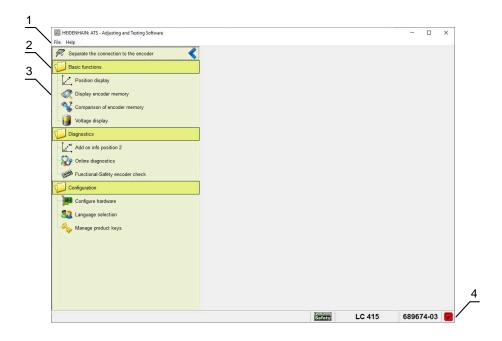
Figure 4: User interface after connecting an encoder
