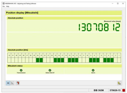
Figure 149: Position display function
