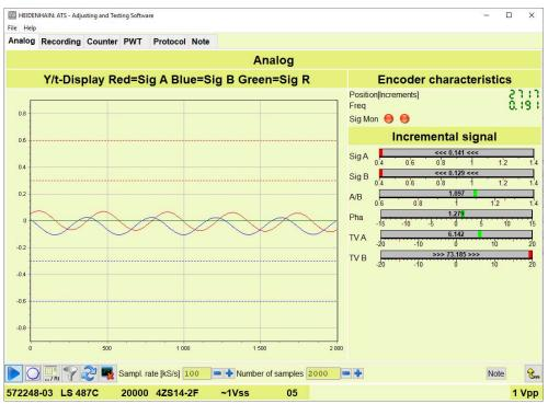
Figure 35: Analog view with Y/t graph
