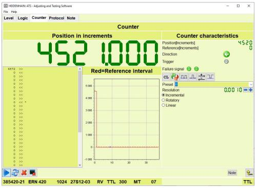
Figure 69: Counter view of the Incremental signal function
