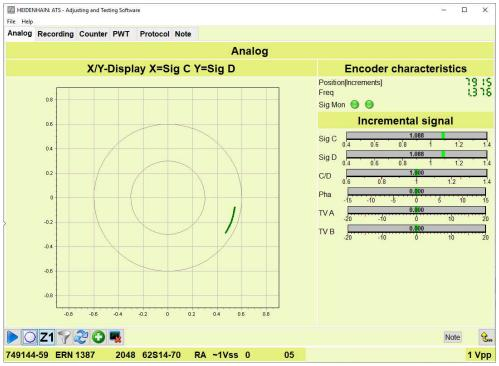
Figure 39: X/Y graph when checking the commutation signals C and D
