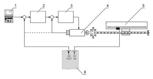
Figure 3: Monitoring mode without signal adapter (no potential segregation)
