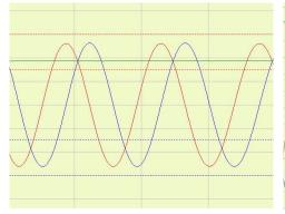
Sufficiently high sampling rate with correct signal shape
