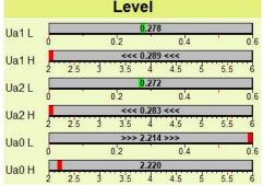
Measured values are within tolerance
