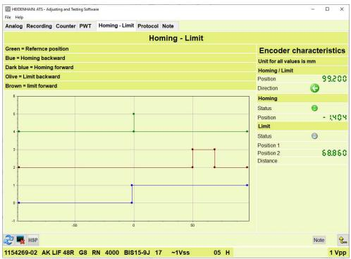
Figure 56: Homing - Limit view of the Incremental signal function
