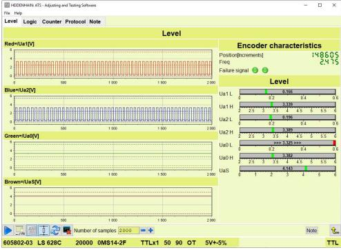
Figure 63: Level view when evaluating inverted signals
