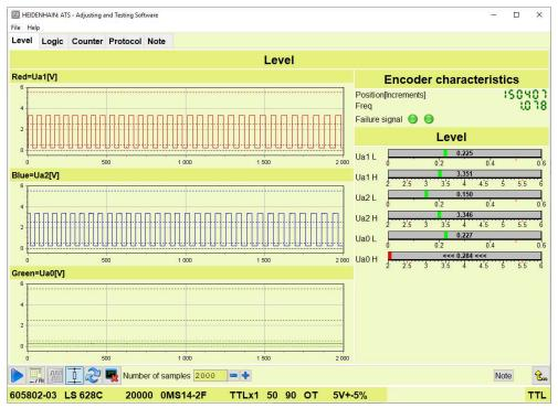
Figure 61: Level view of the Incremental signal function
