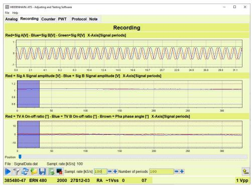
Figure 41: Recording view of the Incremental signal function
