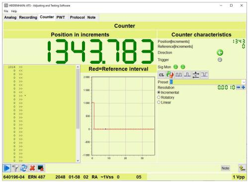
Figure 49: Counter view of the Incremental signal function
