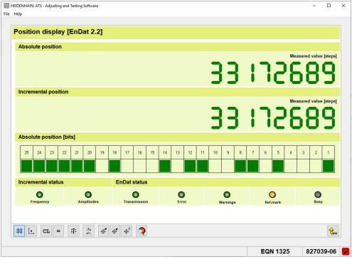
Figure 80: Measured values view of the Position display function
